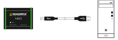
Microsoft® Windows® will install the interface drivers automatically. When ready, the status LED of the device will now fade between red and green.
